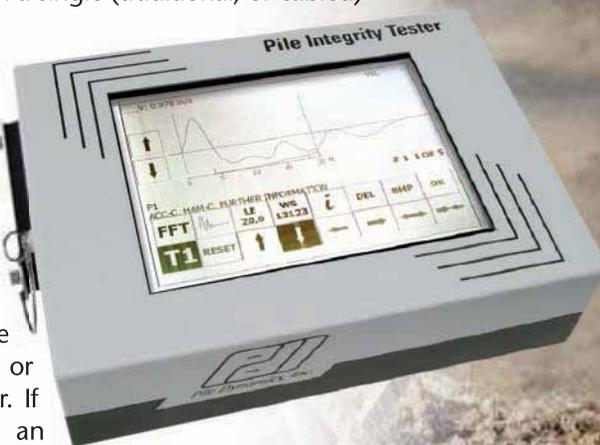
The output of PIT is a graph of the velocity signal versus pile length as shown to the right. Piles with flawless shafts show a reflection from the pile toe as in the augered cast-in-place pile example on right (top). Defective piles show early reflections from the damage location as in the bottom portion of the figure at right. As a rule of thumb, toe reflections should be observed with embedments less than 30 diameters.
